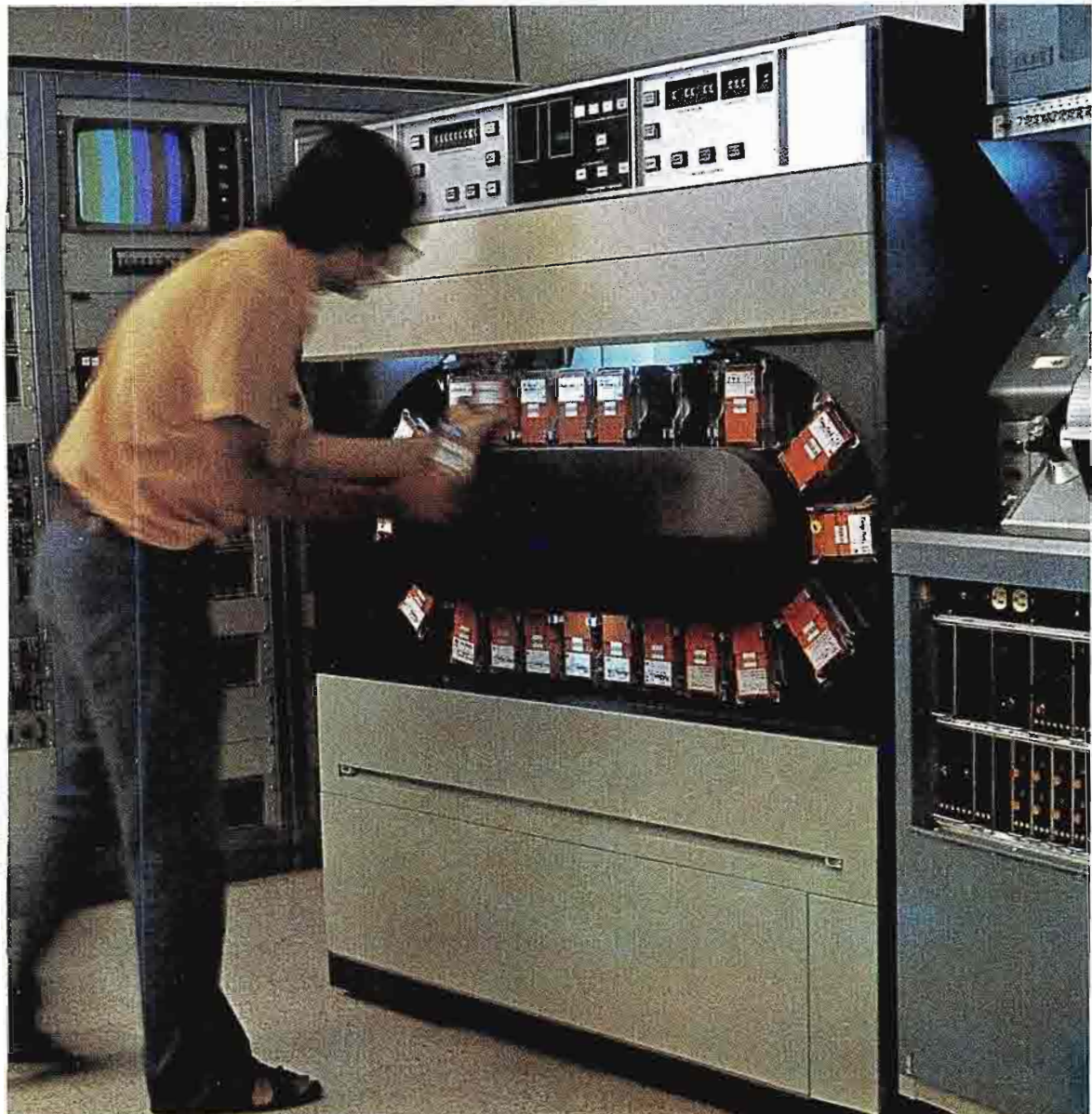
LAST MINUTE CHANGE from traffic is handled easily. Cartridges are exchanged and the new commercial is ready to play.
